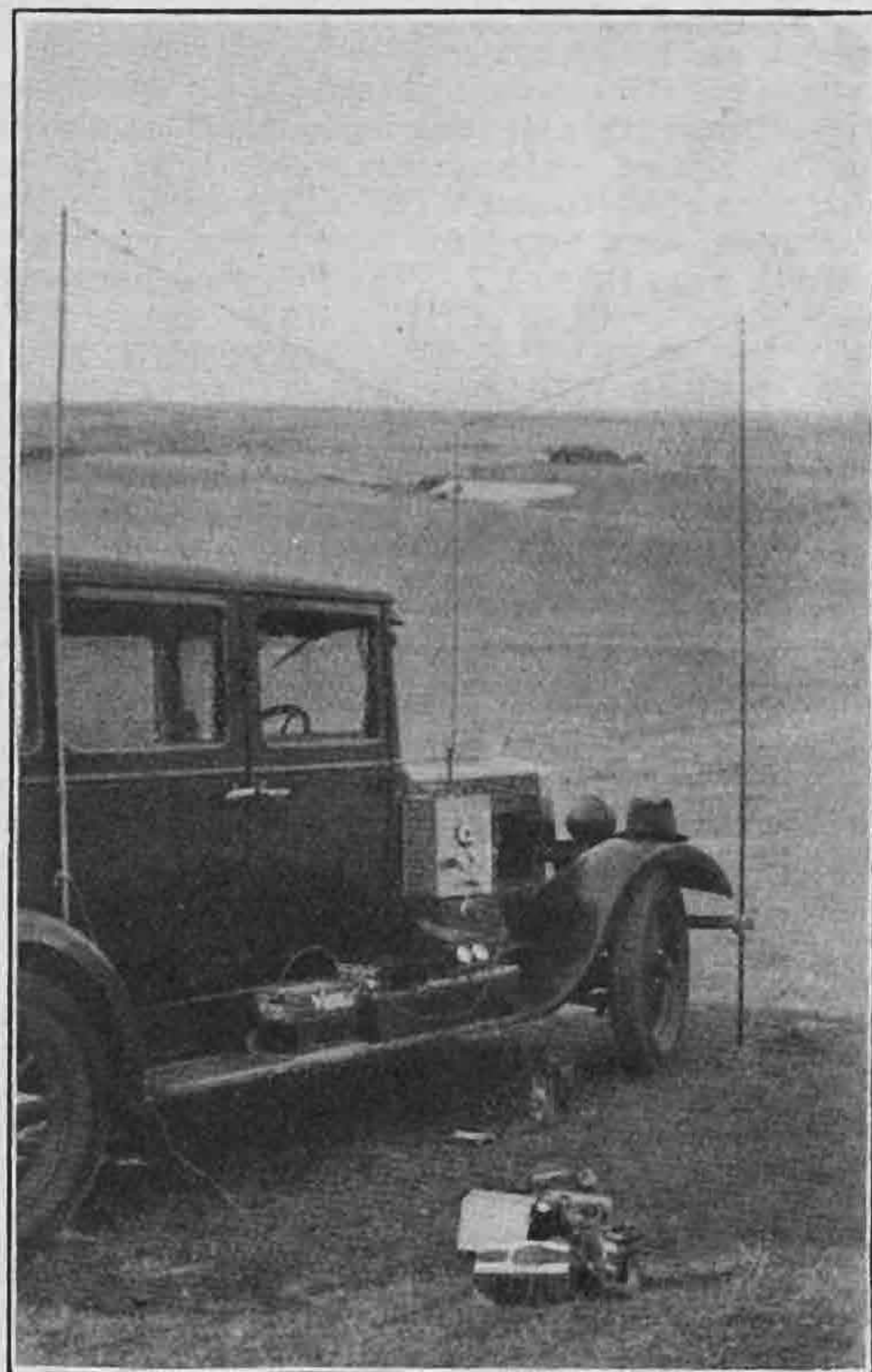
Our photograph shows the receiver and aerial used at the ground station G5CV during the Glider tests. The transmitter is in the aluminium case immediately below the feeder line.
